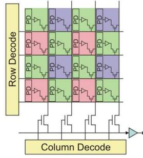
(b) Structure of CMOS sensor
