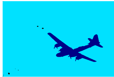
(e) Median3 \times 3 filtered image, with segments containing more than 5% of total pixels extracted
